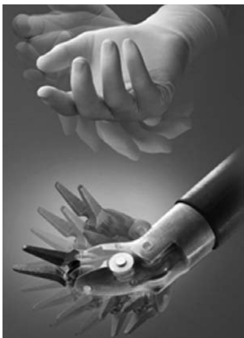
FIGURE 138.5 Wristed instrumentation provides 7 degrees of freedom (left/right, up/down, in/out, rotation, pitch, yaw, open/close).
