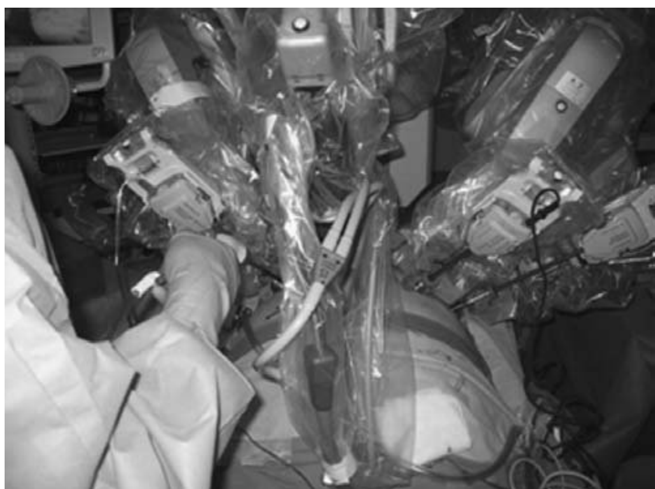
FIGURE 138.6 Bedside assistant's view of the four-arm da Vinci surgical system.
