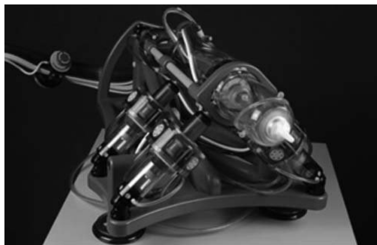
FIGURE 138.1 MrBot, designed for image-guided prostate needle based procedures, is constructed entirely of nonmagnetic materials for MRI compatibility. (Courtesy of Dr. Dan Stoianovici, urobotics laboratory, Johns Hopkins University.)
