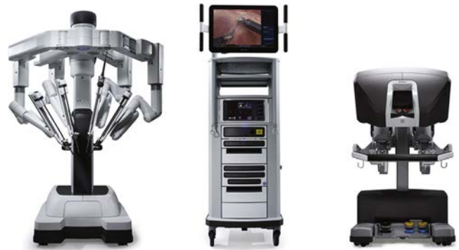
Figure 5-7. da Vinci Xi Surgical System (2014). (Copyright © Intuitive Surgical, Inc., Sunnyvale, Calif.)
