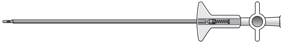
Figure 9-1. Veress laparoscopic insufflation needle.
