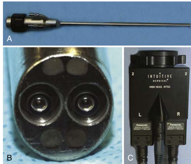
Figure 2-13. Photograph of da Vinci stereo endoscope (A) showing the two individual 5-mm endoscopes (B) and camera (C) with right and left optical channels. (From Higuchi TT, Gettman MT. Robotic instrumentation, personnel and operating room setup. In Su LM, ed. Atlas of Robotic Urologic Surgery, Current Clinical Urology. New York: Humana Press; 2011.)
