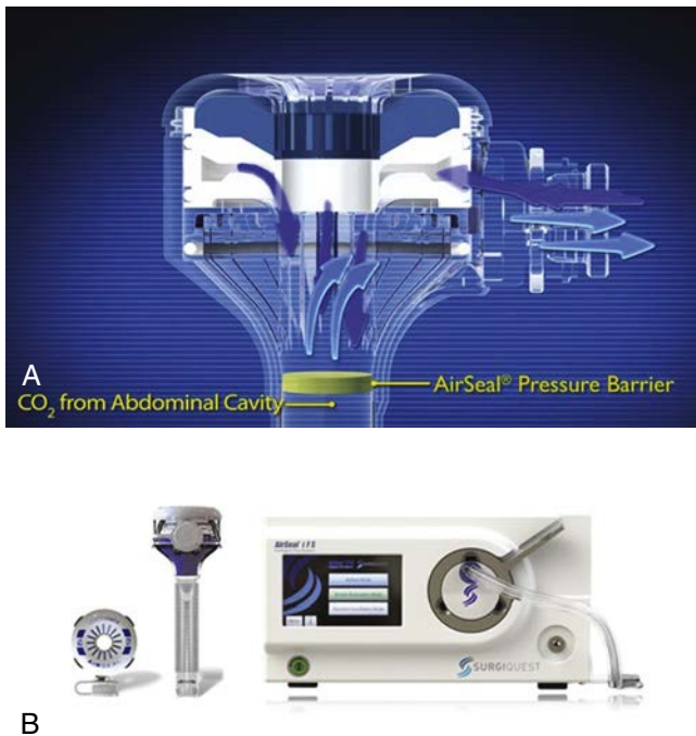
Figure 8-2. A, The AirSeal access port invisible air barrier system. B, A series of high-pressure nozzles directs CO 2 gas downward into the cannula, creating a horizontal air barrier (referred to as a vortex) that maintains desired intra-abdominal pressure. (Copyright © 2015 SurgiQuest Inc., Milford, Conn.)
