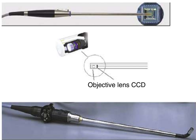
Figure 2-4. EndoEYE technology. This technologic advance allowed for the development of the flexible laparoscope. CCD, charge-coupled device. (Courtesy Olympus America, Melville, NY.)
