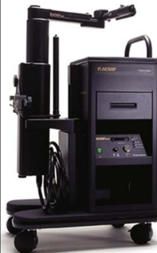
Figure 5-1. AESOP (Automated Endoscopic System for Optimal Positioning) system, a predecessor to the da Vinci Surgical System. (From Regan JJ: Robotics and computers in minimally invasive spine surgery . Spine Universe. Montclair, NJ. http://bit.ly/1MFt8EX .)
