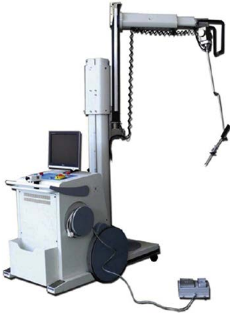
Figure 2-9. First prototype of designed robotic cameraman, RoboLens v1.1, in operational configuration. (From Mirbagheri A, Farahmandi F, Meghdaria A, et al. Design and development of an effective low-cost robotic cameraman for laparoscopic surgery: RoboLens. Scientia Iranica . 2011;18:105-114.)
