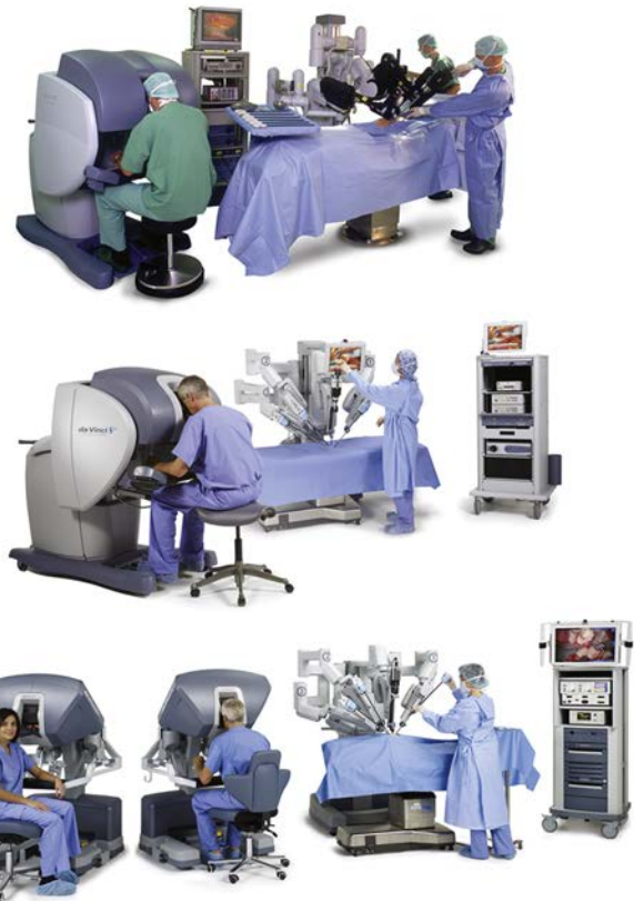
Figure 5-3. Evolution of da Vinci Surgical System: standard model (top, 1999), S (middle, 2006), and Si (bottom, 2009) systems. (Copyright © Intuitive Surgical, Inc., Sunnyvale, CA.)
