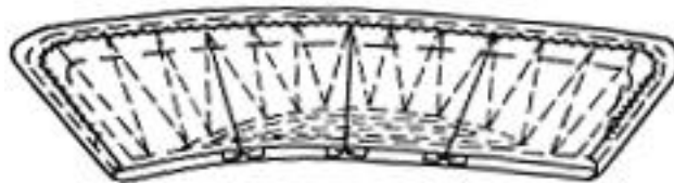
4.29-rasm. Ustki yoqani ostki yoqaga yashirin siniq baxyali maxsus mashinada bostirib tikish.
