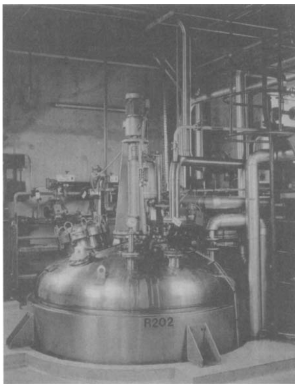
Figure 7.11. Equipment for the production of starter culture concentrate prior to freeze-drying. Note: On-site view of a processing tank for production of starter culture; ammonium compound is used to neutralize the acid produced. (Reproduced by courtesy of Rhodia Food UK Ltd., Stockport, England.)
