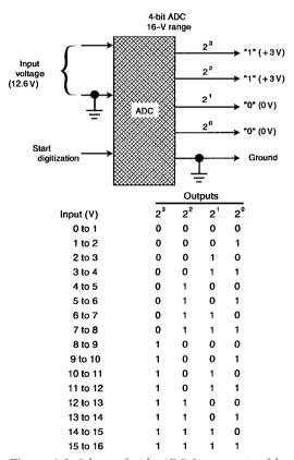
**Figure 4–1.** Scheme of a 4-bit ADC. Inputs consist of the continuous signal to be digitized (range 0– $16\,\mathrm{V}$ ) and a start digitization pulse from a clock that is used to initiate digitization at appropriate times. Outputs consist of four digital signals (+3 or  $0\,\mathrm{V}$  representing "1" and "0") that together can encode a 4-bit integer (range 0–15).
