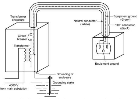
**Figure 2–1.** Scheme of a building's electric power distribution system showing a step-down transformer, circuit breaker, grounding stake, and a third wire for equipment grounding in the conduit. (From Cromwell, L., F. J. Weibell, and E. A. Pfeiffer.1980. *Biomedical Instrumentation and Measurements*, 2nd ed., 437. Englewood Cliffs, NJ: Prentice-Hall. By permission of the publisher.)
