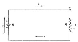
**Figure 1–1.** A simple electric circuit containing an electromotive force,  $\varepsilon$ , current, i, and a resistor, R. The application of Kirchhoff's first law to the circuit starts at point "a." B is a battery (seat of electromotive force) (From Halliday, D., and R. Resnick. 1962. *Physics. Part II, Rev.* 2nd ed., 790. New York: John Wiley & Sons. By permission of the publisher.)
