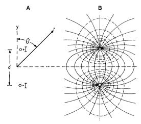
**Figure 3–18.** A current dipole. A, Coordinate system showing definition of r and d. B, Lines of current flow (solid) and equipotential lines (dashed) in a volume conductor. (From Nunez, P. L. ed. 1981. Electric fields of the brain: The neurophysics of EEG. New York: Oxford University Press. By permission of the publisher.)
