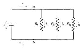
**Figure 1–2.** A circuit containing an EMF,  $\varepsilon$ , and three resistors  $(R_1, R_2, R_3)$  in parallel. a, Junction point (node); b, junction point (node); i, current. (From Halliday, D., and R. Resnick. 1962. *Physics. Part II. Rev.*, 2nd ed., 800. New York: John Wiley & Sons. By permission of the publisher.)
