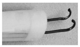
**Figure 45–2.** Hooked electrode that can be used for stimulation or recording from nerves exposed at surgery. The recording surface is exposed along the concavity of the hook. The electrodes are set 10 mm apart.
