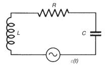
**Figure 1–6.** An AC circuit containing a generator,  $\varepsilon(t)$ , inductor, L, resistor, R, and capacitor, C. (From Halliday, D. and R. Resnick. 1962. *Physics. Part II. Rev.*, 2nd ed., 952. New York: John Wiley & Sons. By permission of the publisher.)
