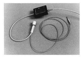
**Figure 21–1.** Etymotic ER-3A transducer, sound tube, ear canal electrode (TIPtrode), and electrode lead. (From Nicolet Biomedical Instruments, Inc., Madison, WI.)
