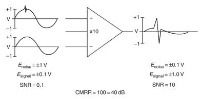
Figure 1–13. A differential amplifier with a small signal on one input and a large artifactual signal on both inputs. The small signal is amplified while the large signal is reduced, but the common mode rejection is not sufficient to totally eliminate the large signal.
