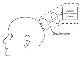
Figure 3–16. A magnetoencephalographic recording device consists of a magnetic field gradiometer (two coils with opposite polarities connected in series) and a SQUID amplifier. (From Nunez, P. L. ed. 1981. *Electric fields of the brain: The neurophysics of EEG.* New York: Oxford University Press. By permission of the publisher.)
