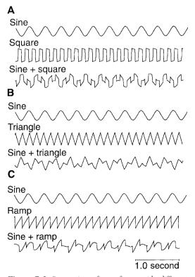
**Figure 7–2.** Summation of waveforms with different shapes but the same frequency (3 Hz) results in more complex waveforms. A sine wave is combined with (A) a square wave, (B) a triangular wave, and (C) a ramp wave.
