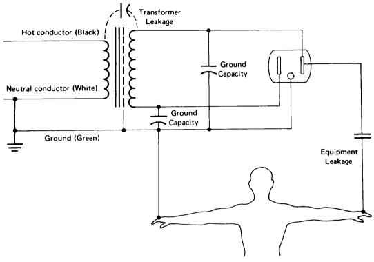
**Figure 2–5.** An isolation transformer used to reduce equipment leakage current. The equipment is connected to the secondary coil of the transformer, which is electrically isolated from the power line hot and neutral conductors. (From Cromwell, L., F. J. Weibell, E. A. Pfeiffer, and L. B. Usselman. 1973. *Biomedical instrumentation and measurements*, 387. Englewood Cliffs, NJ: Prentice-Hall. By permission of the publisher.)
