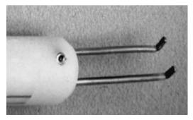
**Figure 45–1.** Bipolar stimulating electrode used for direct stimulation of nerves exposed at surgery. The anode and cathode are separated by a distance of 10 mm.
