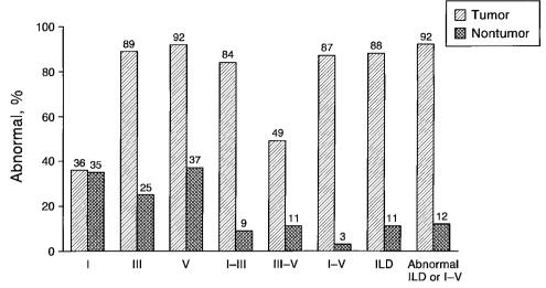
Figure 21–3. Percentage of abnormal (delayed or absent) BAEPs for 75 patients without tumor (nontumor) and 75 patients with CN VIII tumor (tumor) matched for hearing loss. I, III, V, BAEP waves; I–III, III–V, I–V, interpeak intervals; ILD, wave-V interaural latency difference. (From Bauch, C. D., W. O. Olsen, and A. F. Pool. 1996. ABR indices: Sensitivity, specificity, and tumor size. American Journal of Audiology 5:97–104. By permission of the American Speech–Language–Hearing Association.)
