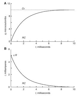
**Figure 1–4.** A, The variation of charge, q, with time, t, during the charging process. B, The variation of current, t, with time, t. For  $R=2000~\Omega$ ,  $C=1.0~\mu f$ , and  $\varepsilon=10~V$ . (From Halliday, D., and R. Resnick. 1962. *Physics. Part II. Rev.*, 2nd ed., 804. New York: John Wiley & Sons. By permission of the publisher.)
