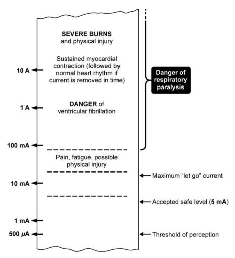
**Figure 2–2.** Effects of 60 Hz AC electric current flow of various magnitudes produced by a 1-second external contact with the body. (From Cromwell, L., F. J. Weibell, and E. A. Pfeiffer.1980. *Biomedical instrumentation and measurements*, 2nd ed., 434. Englewood Cliffs, NJ: Prentice-Hall. By permission of the publisher.)
