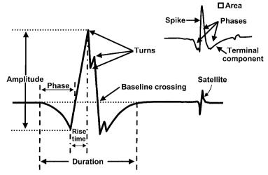
Figure 27-4. Commonly measured variables of the MUP.
