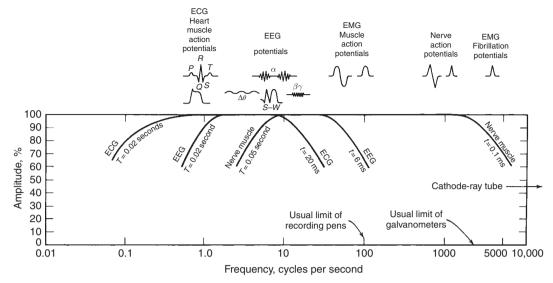
Figure 7–3. The frequency components of electric activity recorded in clinical neurophysiology are shown on a logarithmic scale. T and t are the upper and lower time constants of each frequency cutoff. ECG, electrocardiogram; EEG, electroeacephalogram; EMG, electromyogram. (From Geddes L. A., and L. E. Baker. 1968. *Principles of applied biomedical instrumentation*. 317. New York: John Wiley & Sons. By permission of the publisher.)
