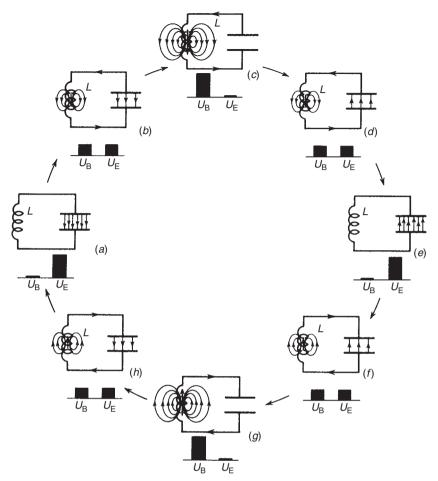
**Figure 1–5.** A simple LC circuit showing eight stages (a-h) in one cycle of oscillation. The bar graphs under each stage show the relative amounts of magnetic  $(U_{\rm B})$  and electric  $(U_{\rm E})$  energy stored in the circuit at any time. (From Halliday, D., and R. Resnick. 1962. *Physics. Part II. Rev.*, 2nd ed., 944. New York: John Wiley & Sons. By permission of the publisher.)
