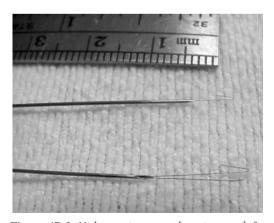
**Figure 45–3.** Nichrome intramuscular wires used for intramuscular EMG recordings. The wire sits inside the core of a small hypodermic needle. The needle is used to insert the wire into the muscle. The wires remain in places after the needle is withdrawn.
