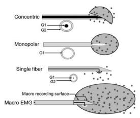
**Figure 26–2.** Electrode types used in recording EMG signals. The recording areas of each electrode type are shown by the hashed regions.
