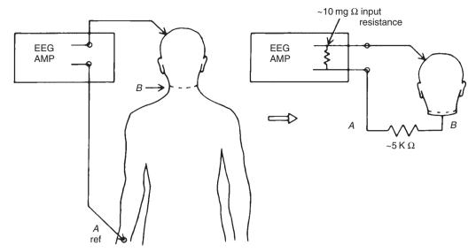
**Figure 3–14.** The futility of using a distant reference for scalp EEG recording. The right arm reference (A) is electrically equivalent to a neck reference (B), except for a slight additional resistance in series. AMP, amplifier. (From Nunez, P. L. ed. 1981. *Electric fields of the brain: The neurophysics of EEG*. New York: Oxford University Press. By permission of the publisher.)
