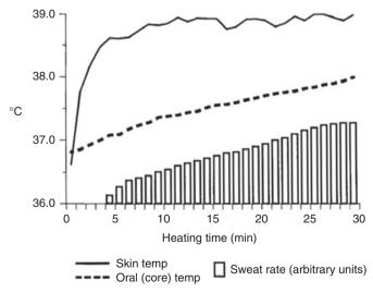
**Figure 38–4.** Mean skin and oral temperatures and sweat rates of 35 healthy controls during the TST. By 38°C oral temperature, all had reached a maximum sweat rate. (From Fealey, R. D. 1997. Thermoregulatory sweat test. In *Clinical autonomic disorders: Evaluation and management*, ed. P. A. Low, 2nd ed., 245–57. Philadelphia: Lippincott-Raven, Figure 2.)
