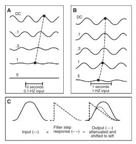
**Figure 1–9.** A high-pass filter shifts the latency of lower frequency waveforms more than higher frequency. Note the greater effect on the 0.1-Hz waveform than on the 1.0-Hz waveform.
