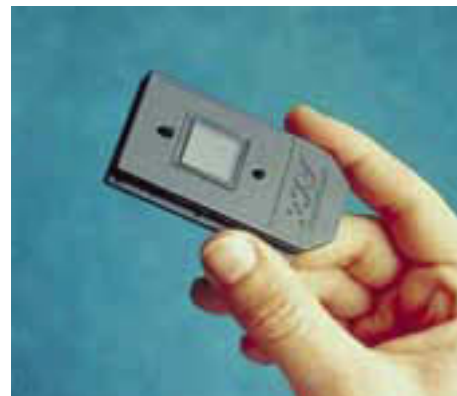
Figure 17.16 Affymetrix GeneChip® probe array (courtesy of Affymetrix)
