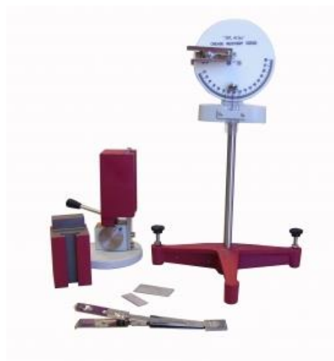
1.81-rasm. M003A SHIRLEY CREASE RECOVERY TESTER & LOADING DEVICE asbobi.
