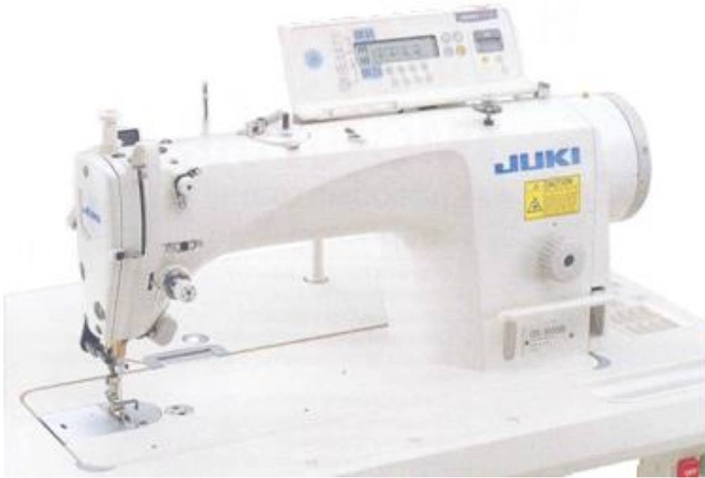
1.19-rasm. “Juki” firmasining moki baxyali universal tikuv mashinasi
